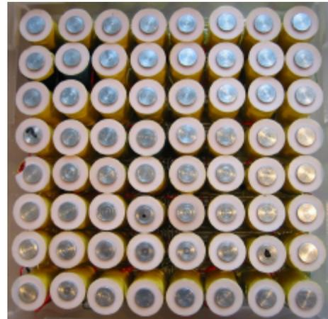
Figure 3: Overhead view of electromagnet array.
