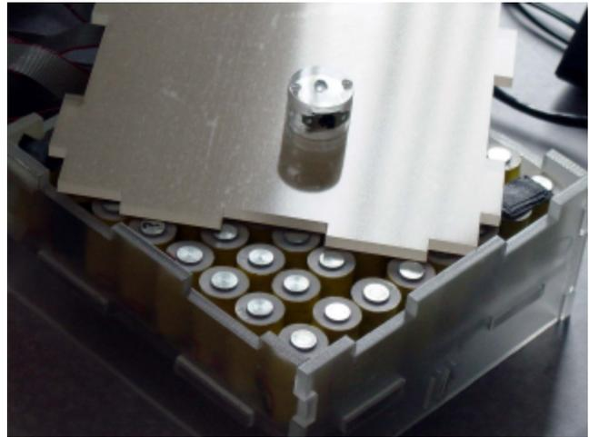
Figure 1. The Actuated Workbench uses a grid of electromagnets to move a magnetic puck across a table surface.
